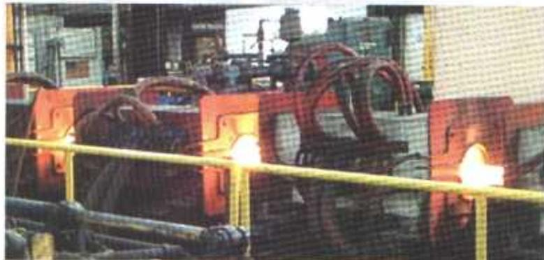
*As is typical for most in-line production systems with frequent up and down times, operating costs are reduced since no holding temperatures are required during idle time.*
