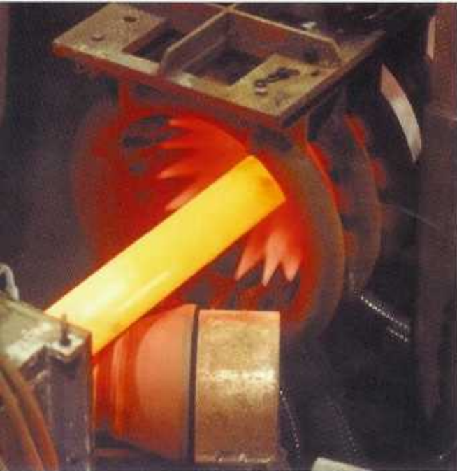
Ajax TOCCO Magnethermic quenching system installed on an austenitizing and temper line for the production of high strength casing and tubing. ERW pipe is quenched to essentially a full martensitic structure then tempered.
