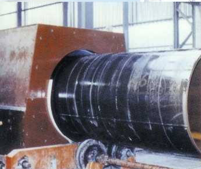
Ajax TOCCO Magnethermic wide oval cast coil for heating 6 to 12 strands of rebar prior to fusion bond epoxy coating.
