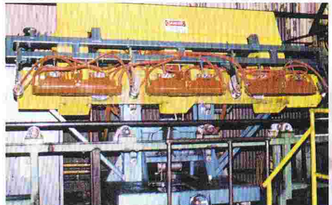
Multiple inductors mounted on a common base allow for high kilowatt applications with limited floor space. Guide rolls located at each end of the fixture and between each inductor control the pipe to inductor gap insuring efficient operation.
