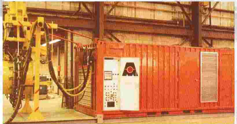
Portability is the key to weld annealing in the field. Here all the equipment necessary to weld anneal 42" diameter pipe is contained and mounted on a skid for on location use. The inductor is a hydraulically operated split design, which operates as a clam shell to fit precisely over the weld area in the installed pipe line.
