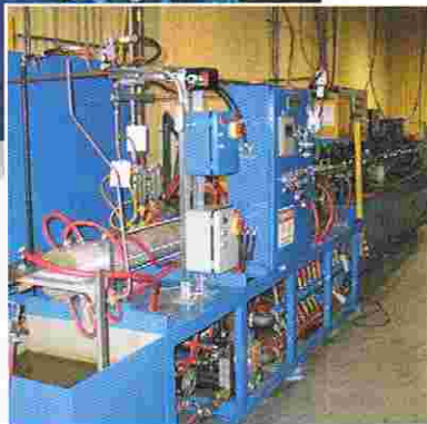
Solution anneal heat treatment is used to restore both corrosion resistance and ductility to hot worked tubing. An Ajax TOCCO Magnethermic system provides controlled heating and cooling to dissolve carbides and control grain growth.
